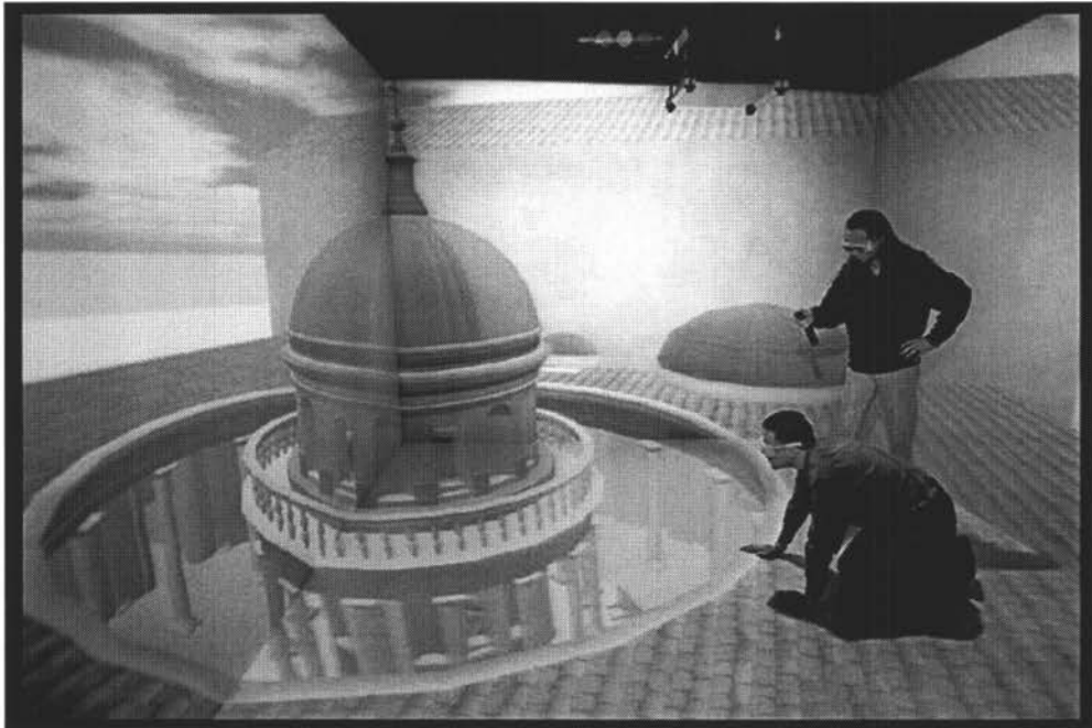
Figure 4 Multiple Immersive Projection Systems (CAVE-like systems)
